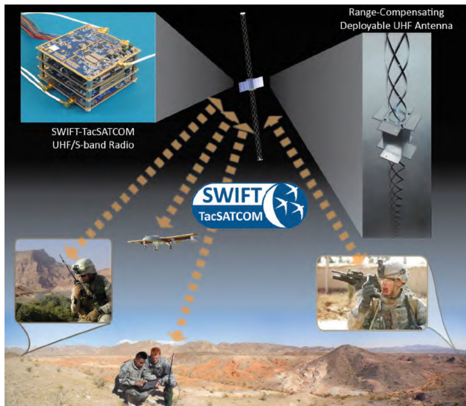
Caption: Tethers Unlimited’s SWIFT-TacSATCOM radio system enables tiny CubeSats to communicate directly with standard handheld UHF radios used by soldiers in the field.
