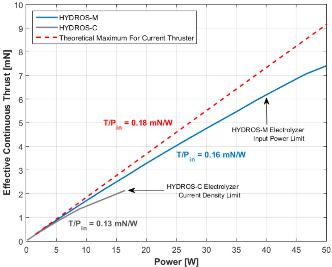
**Figure 9. HYDROS Effective Continuous Thrust**
