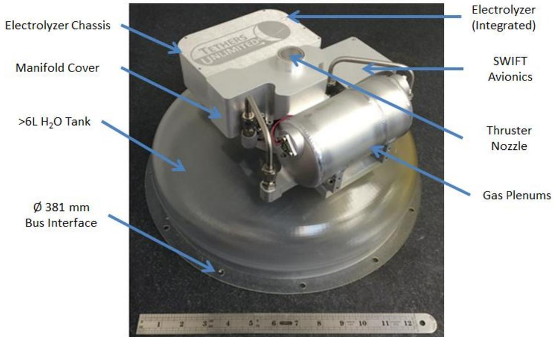
**Figure 3. HYDROS-M Propulsion System.**
