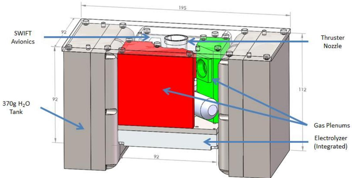
**Figure 2. HYDROS-C Thruster with 740 g Capacity 'Saddlebag' Tank Configuration (mm).**
