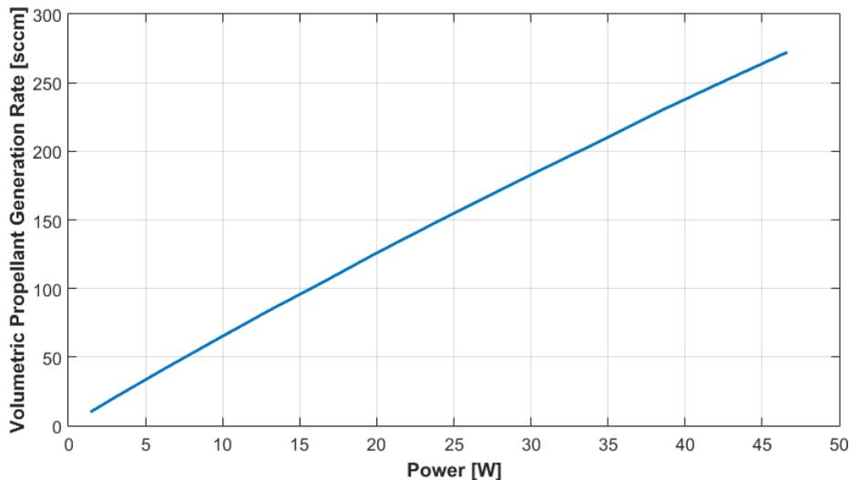
Figure 4. HYDROS-M Electrolyzer Performance Testing Results
