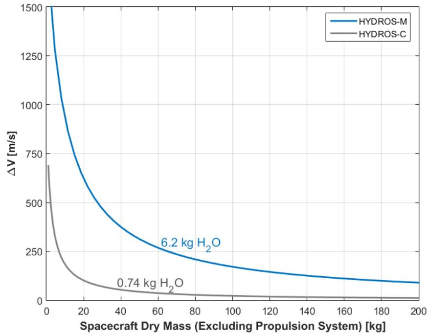
**Figure 8.  $\Delta V$  Delivered by the HYDROS-C and HYDROS-M Thruster Variants Across a Range of Spacecraft Masses**
