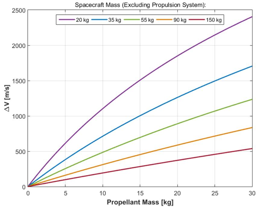
**Figure 7.  $\Delta V$  Delivered by HYDROS-C Thruster with Expanded Water Tank(s) Across a Range of Spacecraft Masses**
