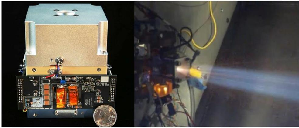
**Figure 1. HYDROS-C Engineering Unit (left) Being Tested in a Vacuum Chamber (right).**
