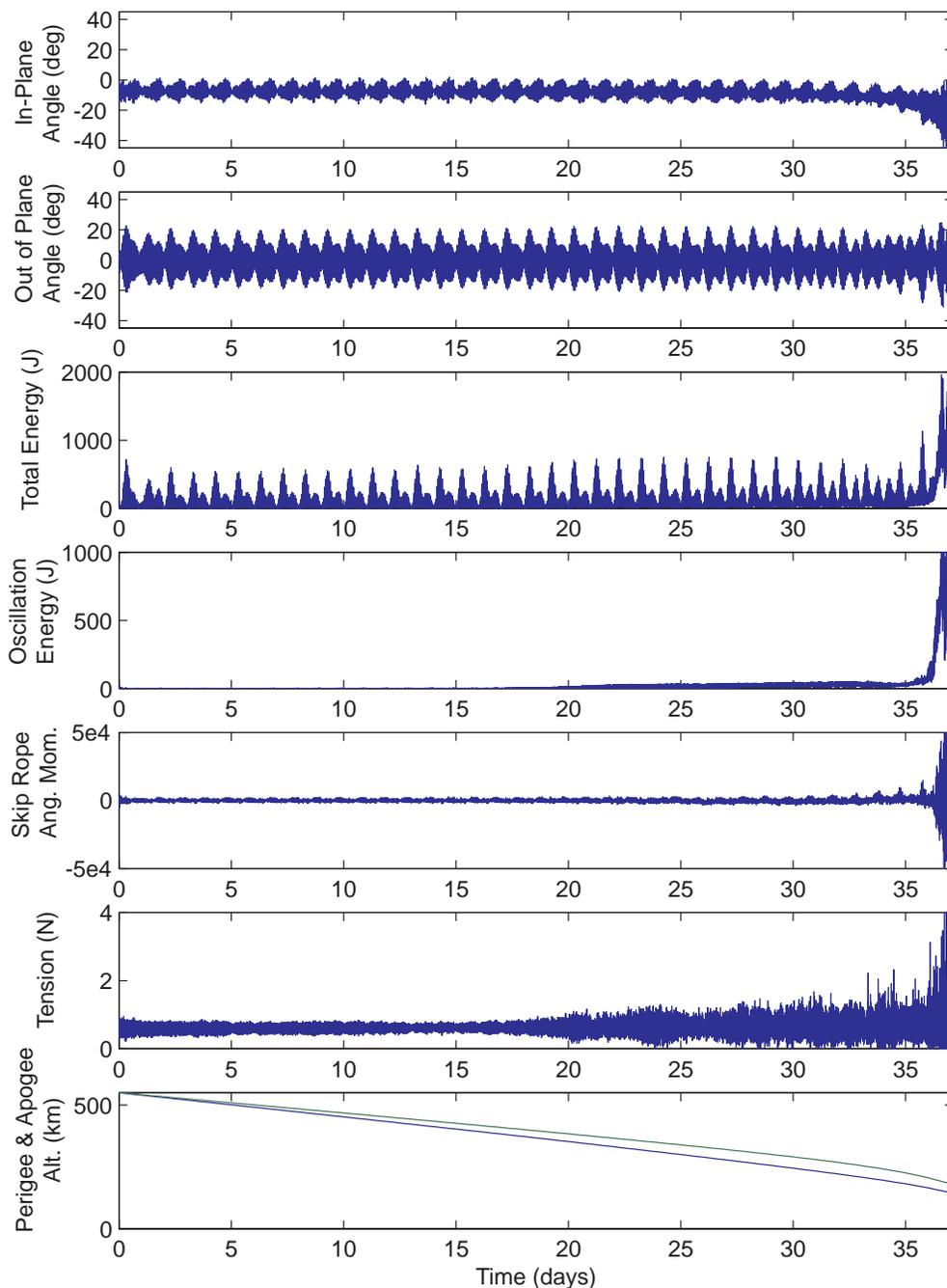
Figure 5. Simulation of deorbit of the GLAST spacecraft, with feedback control on both oscillation modes and in-plane libration. Tether only loses stability after it enters the upper atmosphere.
