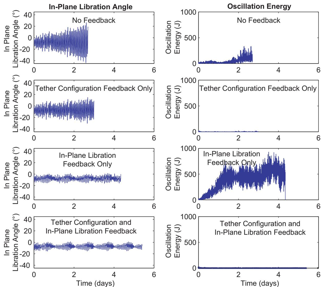
Figure 3. Comparison of simulation results for deorbit of a 3360 kg GLAST spacecraft by a Terminator Tether™ device with a 15 kg, 10 km tether and a 15 kg endmass, with no feedback, tether configuration feedback, in-plane libration feedback, and both tether configuration and in-plane libration feedback.
