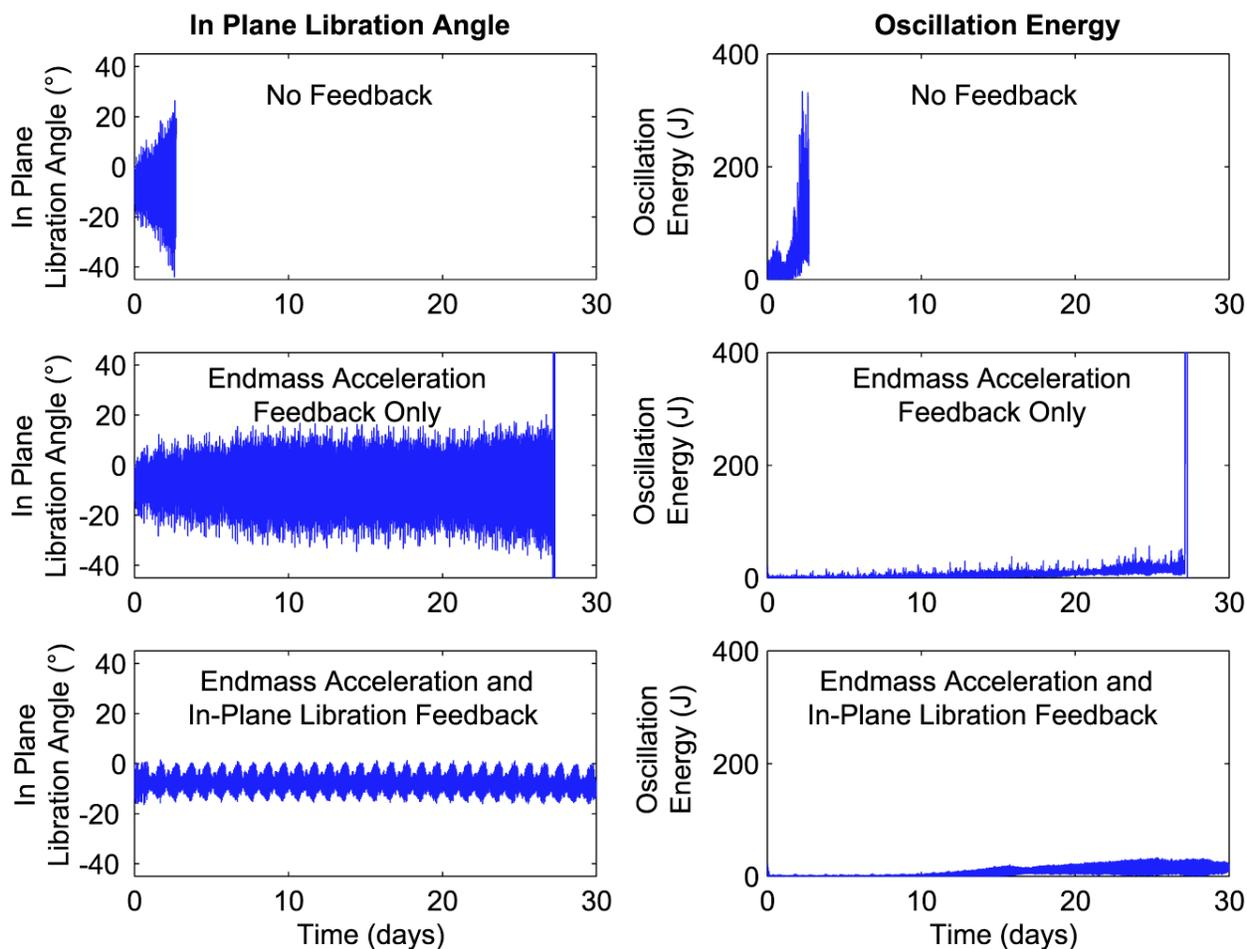
Figure 4. Simulation results for deorbit of the 3360 kg GLAST spacecraft using a Terminator Tether™ with a 15 kg, 10 km long tether and a 15 kg endmass, with and without feedback based on the endmass acceleration.
