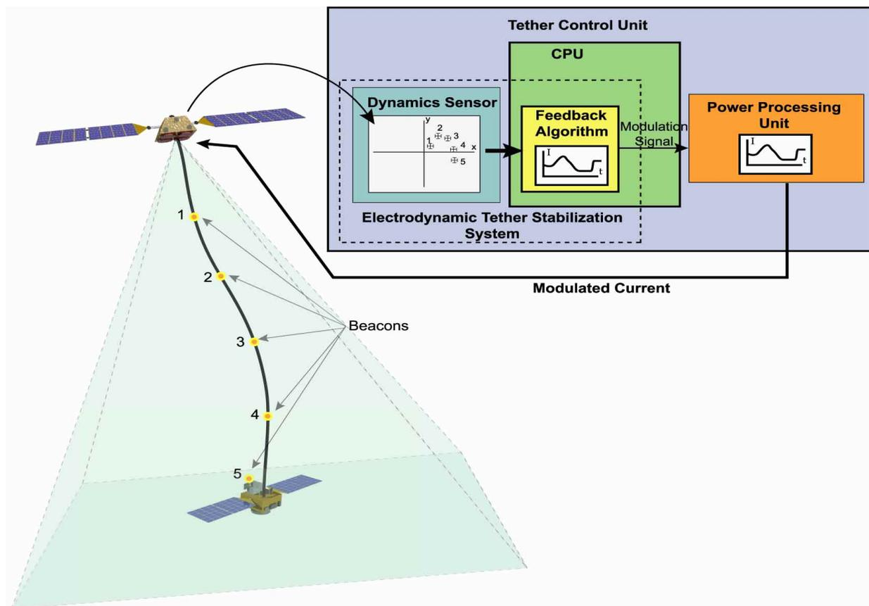
Figure 2. The Electrodynamic Tether Stabilization (EDTS) System.
