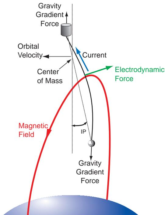
Figure 1. Electrodynamic tether, in drag mode.
