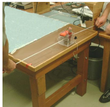
Figure 4 Tether inspector conceptual design and proof-of-concept demonstration.
