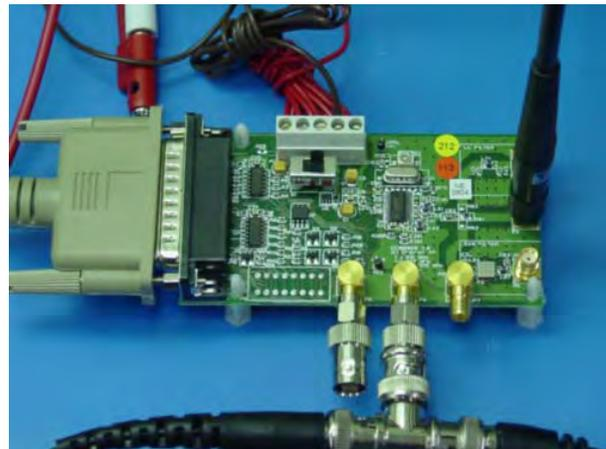
**Figure 15: Communication System Prototype - Chipcon CC1000 Development Board.**
