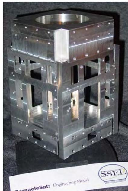
**Figure 13: BarnacleSat Structure Engineering Model**
