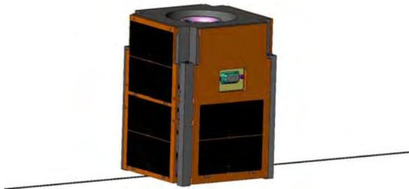
**Figure 18. Rendering of the external view of BarnacleSat.**
