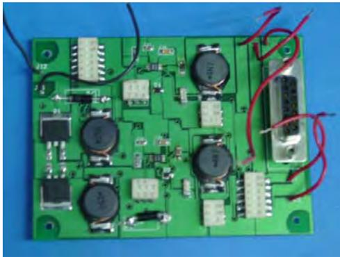
**Figure 16: 5V Regulator, Test Board**
